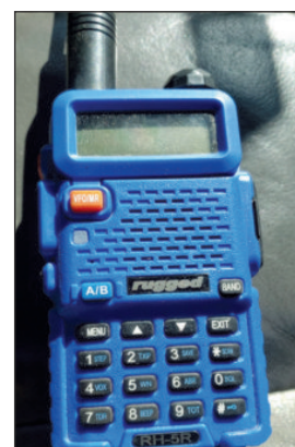
Race teams communicate with their support crews and with race officials via handheld radios such as this. Cell phones are worthless over much of the course.
