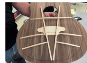
Revolutionary "V" bracing beneath top board. Taylor has the patent for 10 years
