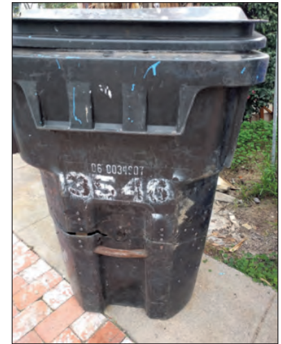
Screws on the outside, wood on the inside keep this one together
