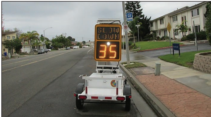
Oceanside's fake speed cameras do not record anything but speed data for traffic engineers.
