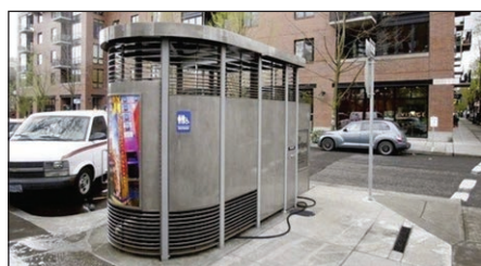
The three-ton stainless-steel Portland Loos use less than a gallon and a half per flush.
