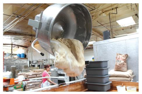
A mixing-bowl lift drops 300 lbs. of dough onto a table. The dough is then cut and sent to a temperature-controlled proofing room, where it will rise.
