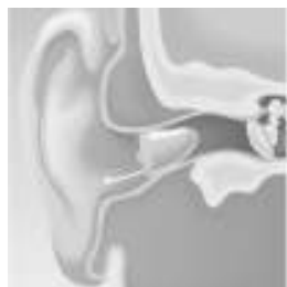
Conventional hearing aids can "plug-up" the ear canal creating a "barrel effect" to the wearer.
