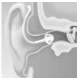
HearStic uses a vented ear bud, which allows natural sounds to pass through without amplification.
